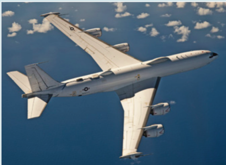
A second angle on a VX-20 E-6B conducting flutter testing.
